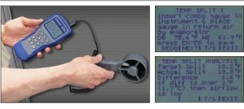
Just two measurements with the probe will give the target temperature split and actual temperature split across the evaporator and compare the two.
